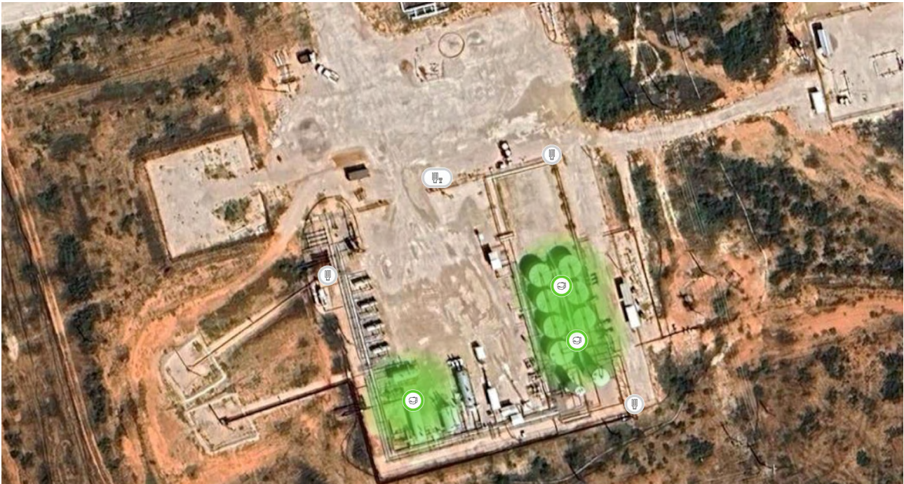
Figure 3: Deployment example of three Nubo Sentry sensors covering key equipment in addition to Nubo Sphere for fenceline monitoring.
