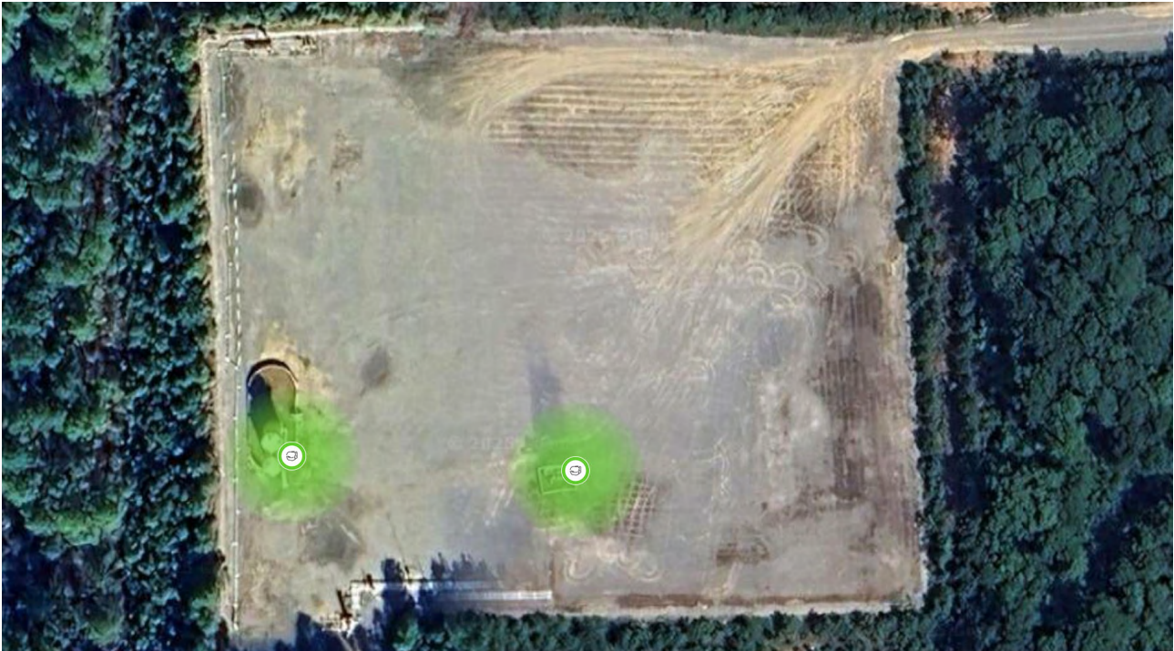
Figure 2: Deployment example of two Nubo Sentry nodes covering a simple site for reliable, low-cost methane monitoring.
