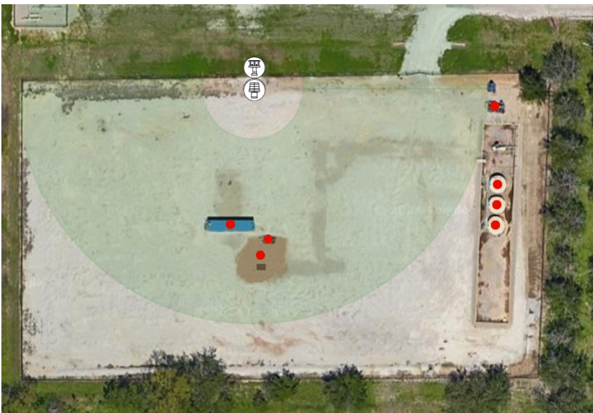
Figure 5: The wind rose indicates that prevailing winds are from the south and likely to carry emissions to sensors placed north of sources. One sensor node is, therefore, placed on the north fence line. But it can only cover some of the equipment on this site. The Nubo Sphere siting procedure has labeled sources with dots, indicating inadequate source coverage.
