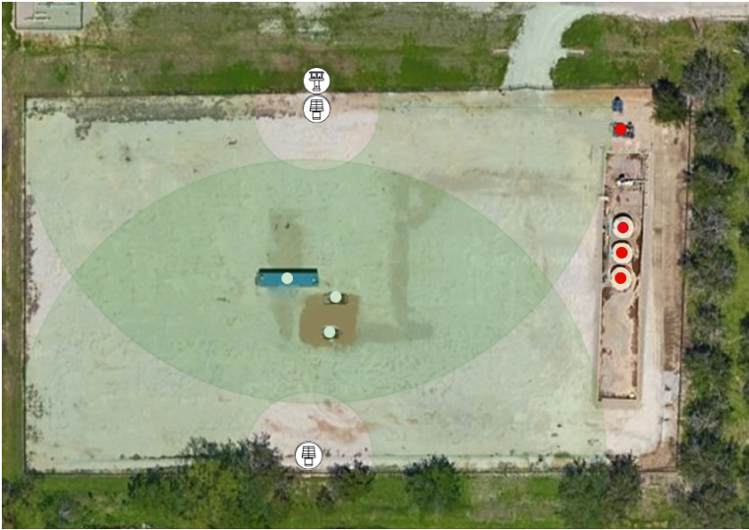
Figure 6: Adding a second sensor node improves coverage of the equipment in the center of the site. White dots labeling this equipment indicate good coverage. Source coverage has improved. The sources on the eastern edge of the site, however, remain out of sensor range.
