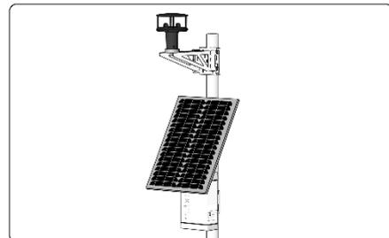
4. For ease of installation, the mounts are designed so that the node and the accessories remain in place without the screws being tightened. However, it is important to tighten the screws on the side to ensure safe and secure fixation of the system under all weather conditions. Do not overtighten the screws.
