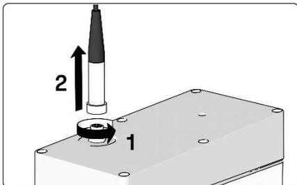
Unplugging the cable will turn off the device and disconnect the battery for transport. After the device has been powered down, be certain to correctly install the protective cap to protect the pin's connector and avoid corrosion or dirt build-up.
