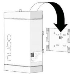
3. Mount the sensor node to the lower plate and the solar panel to the upper plate.
