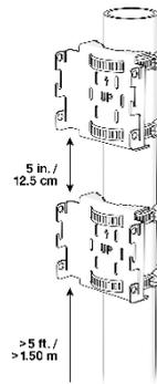
All plates should face the orientation of the sun at noon. The plates should therefore face south in the Northern Hemisphere and north in the Southern Hemisphere.
