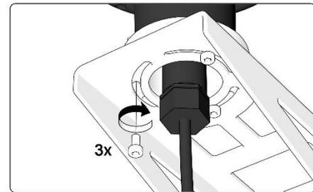
8. Connect the solar panel to the cable power plug on top of the sensor node. **Make sure to properly align the connector to the socket, and not to force the connection. A miss-plugged cable will prevent charging of the battery.** Always tighten the union nut to ensure proper protection from water ingress.
