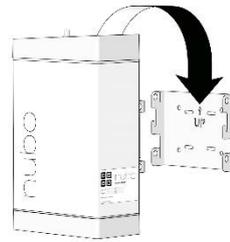
3. Mount the sensor node to the bottom plate, the solar panel to the middle plate and the wind meter arm to the upper plate.
